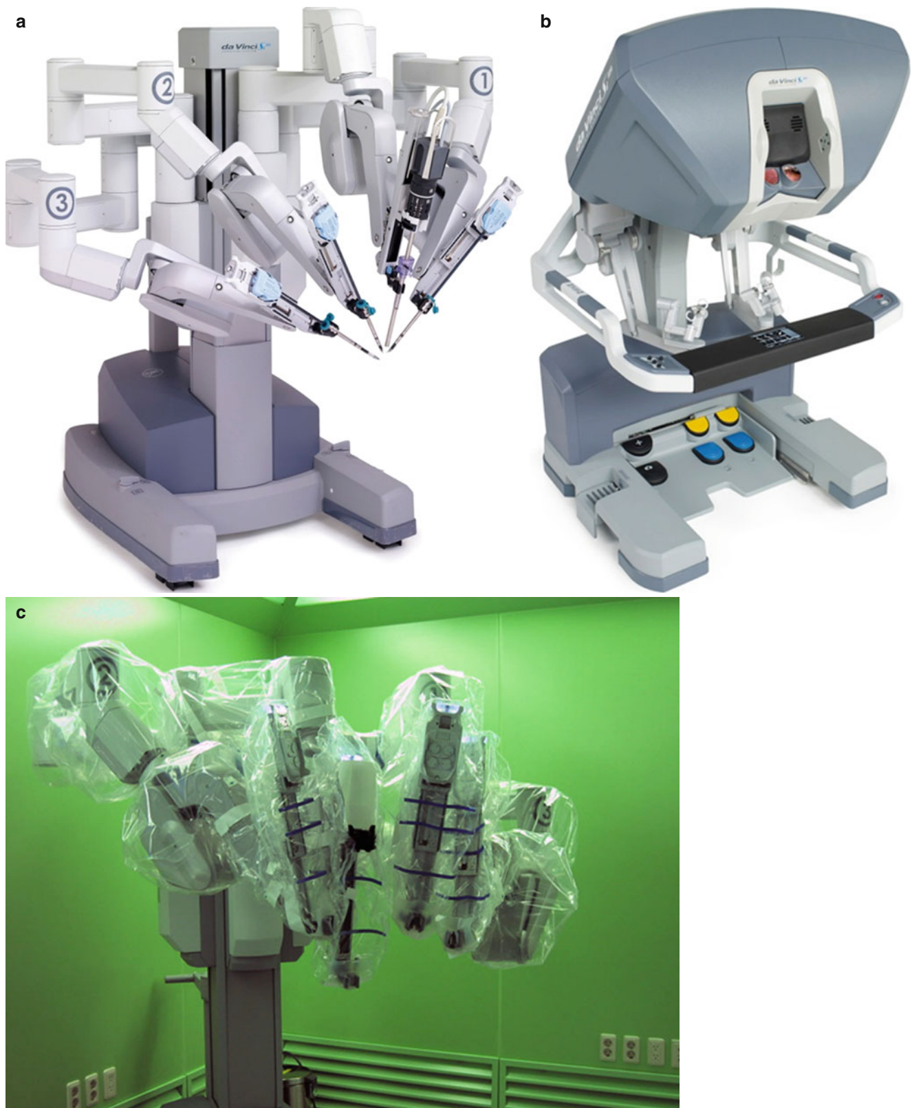
Fig. 4.1 The da Vinci system. (a) Robot system, (b) console, (c) da Vinci system before use
