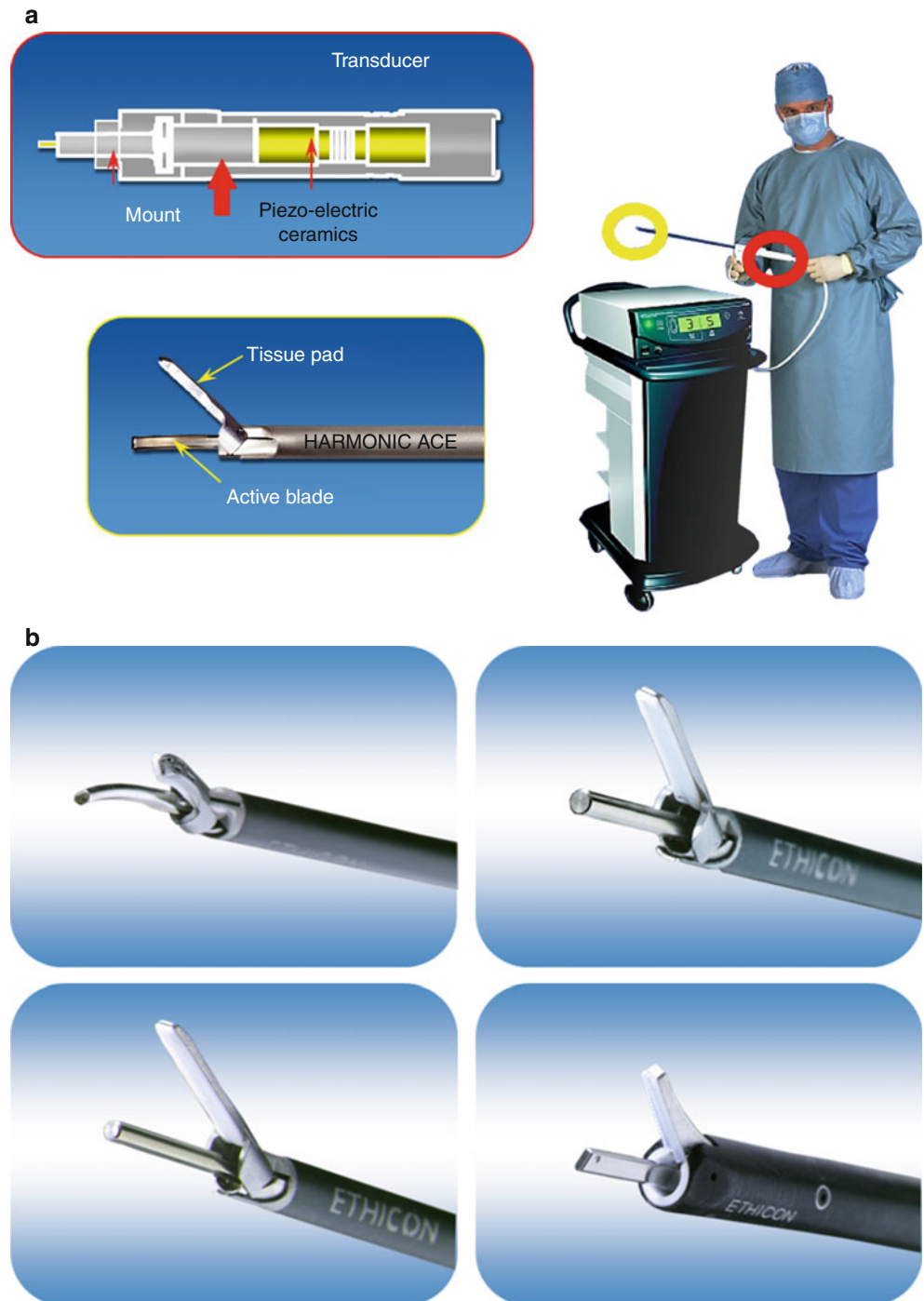
Fig. 6.2 Harmonic® shears (Image courtesy of Ethicon Endo-Surgery). (a) The transducer generates ultrasonic vibration that makes an active blade vibrating 55,500 times a second. This mechanical energy allows simultaneously cuts and coagulates tissue, (b) various types of the tips
